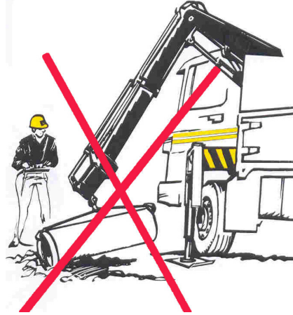
Figure 8.11: Never drag a load sideways
