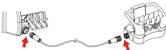
Figure 3.4: Cable remote control
