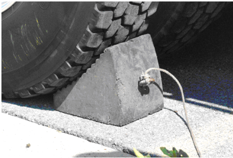
Figure 7.6: Setting wheel chocks
