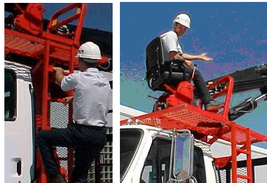
Figures 3.5a & 3.5b: Top Seat Control Station
