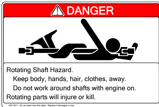
Figure 2.7: Rotating Shaft Hazard decal (A07)
