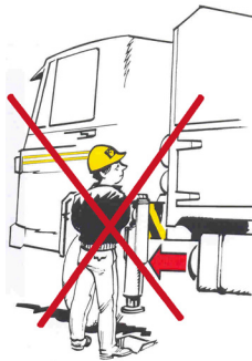
Figure 7.11: Stay away from stabilizer beams when they are moving
