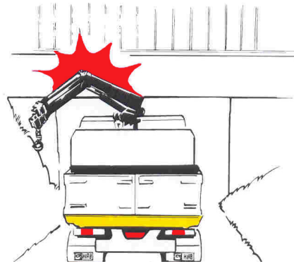
Figure 8.14: Always travel with the crane properly stowed.
