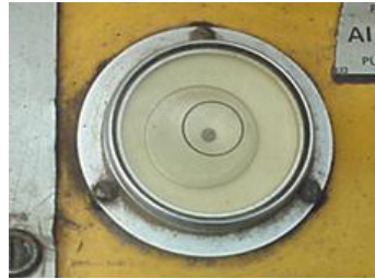
Figure 7.15: Sample bull's eye level
