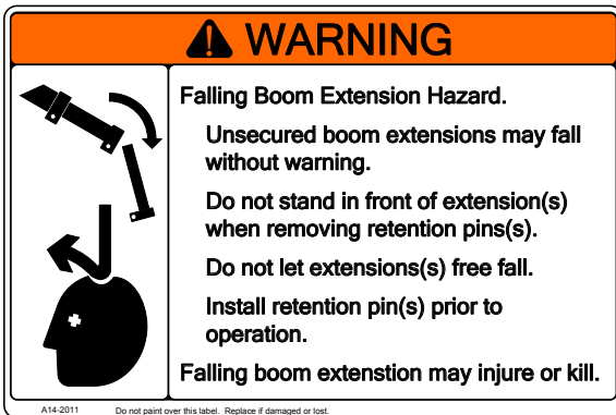
Figure 2.14: Boom Extension decal (A14)
