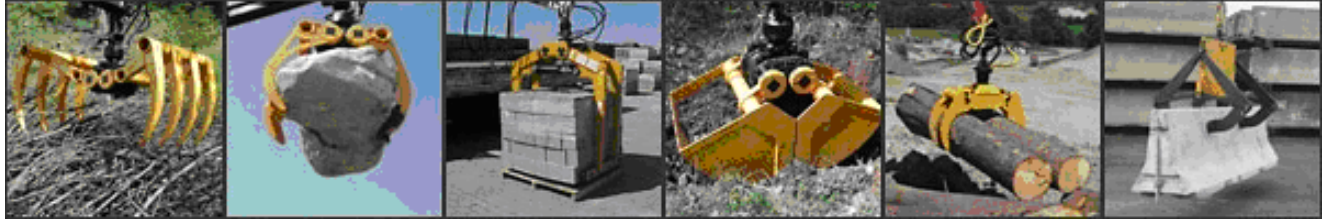
Figure 4.1: Typical articulating crane attachments
